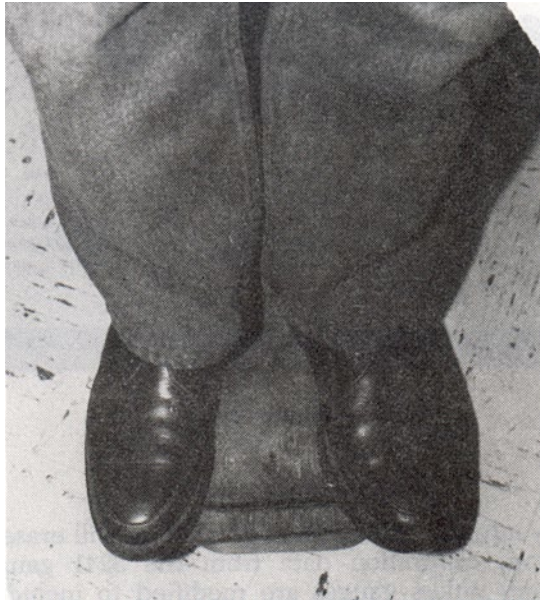
FIGURE 3. Standing on Pressing Board for Compaction
